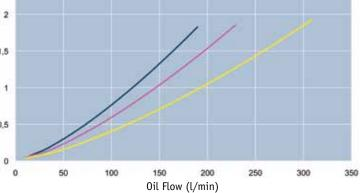
Inlet oil temperature 60°C at  $\Delta p$  max 2 bar Inlet water temperature 20°C
